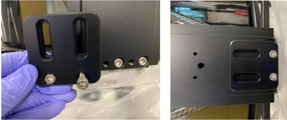
Figure 6. Install Scope Stopper (X2) onto scope Losmandy bar (front ends)
